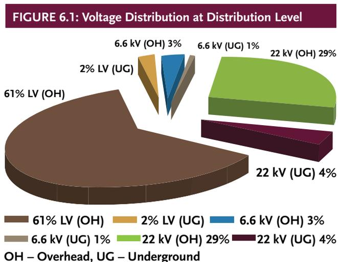
The distribution network consists of overhead lines and underground cables. In town centres, such as Port Louis, Curepipe, Vacoas, Quatre Bornes and Rose Hill, and where access to the construction of an overhead network is not practical, underground cables are used.
